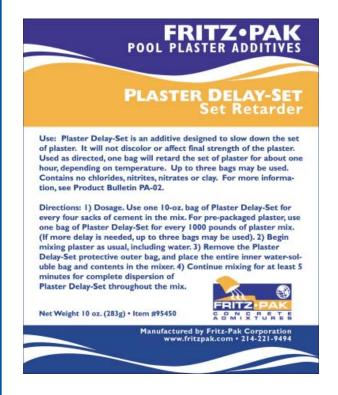
as directed, one bag will retard the set of plaster for about one hour, depending on temperature. Up to three bags may be used. Contains no chlorides, nitrites, nitrates or clay.
